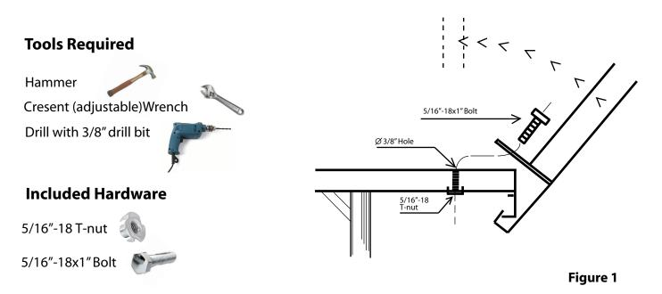
**Step 1:** Put the guard rail on the stage in the desired position. Hook it onto the edge of the stage platform and rotate it up into place as pictured in Figure 1.
