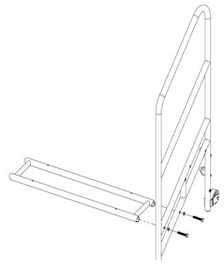
Begin by aligning one of the sides of the metal step frame to the inside of one of the guardrails. Important: Make sure that the side of the metal step frame is marked the same as the guardrail.
