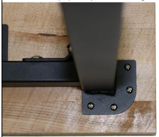
**TO ADJUST LEG HEIGHT**—Use the allen wrench (Part D) to remove the two allen screws and lock-washers from the bottom side of each upper leg. Once removed, slide the lower leg to your desired height and then re-fasten the allen screws with lock washers to each upper leg.
