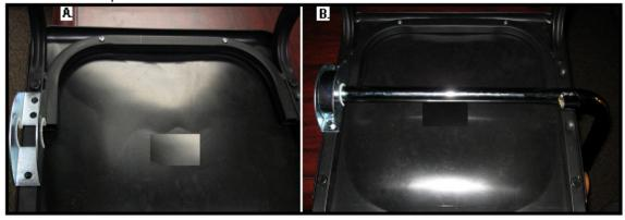
5. Before attaching bracket and bracket cover on the right side, lift arm to the position in the below picture. Attach bracket and bracket cover to the frame of the chair using a ratchet with a \_" socket. IMPORTANT: Make sure to place bracket on frame with the two holes facing front of chair as shown below.
