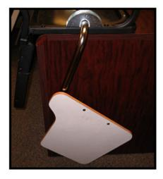
7. Insert the hex-head screw through the hole of the bracket on the right side using a 7/16" ratchet. Place lock nut on and tighten with a pair of pliers.
