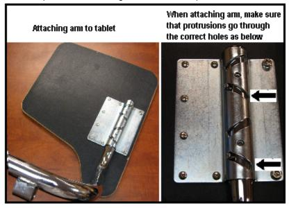
3. Tighten bolts with nuts using a 7/16" socket. Screw in the six screws with a Philip screwdriver.
