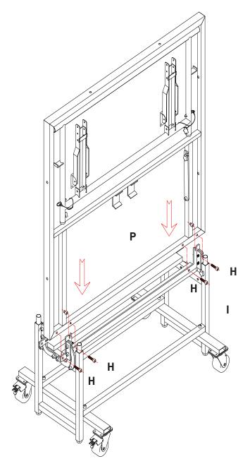
5. Insert stage platform P into the base I and secure it with allen screws H
