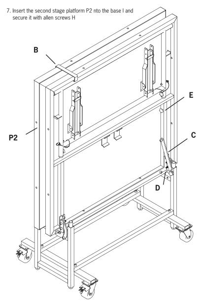
8. Install safety lock B to secure top of stage platfroms together for safety
